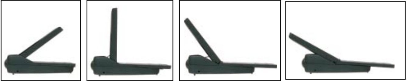
The innovative keyboard hinge on the Psion 5 moves the weight forward so the machine doesn't tip over when you tap the screen
